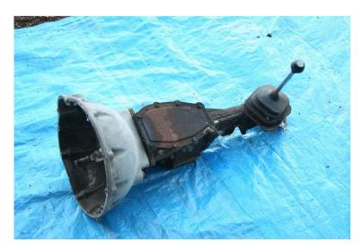
4-speed manual gearbox (goes with 6-cylinder motor)
